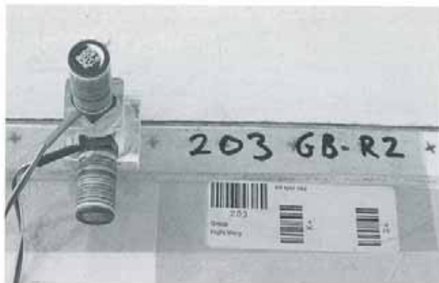
Fig. 7: The use of bar codes, nonresidue tape, and hot glue enhances the accelerometer installation
