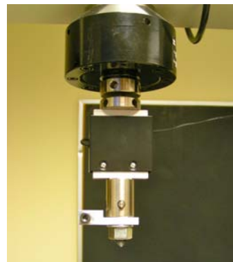
Fig. 30 Load cell setup for QMT bending stiffness tests.
