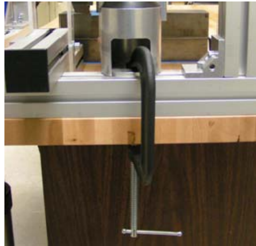
Fig. 47 A C-clamp is used to secure the humerus clamp to the MRTA table.
