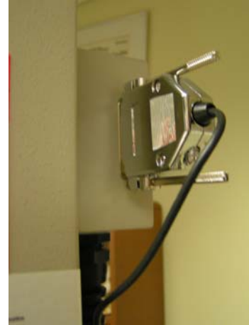
Fig. 31 D-Connector attachment for 25 N load cell
