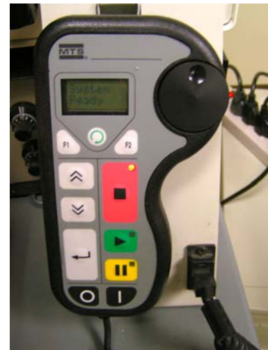
Fig. 22 QMT Remote control used for adjusting the crosshead and turning on the device
