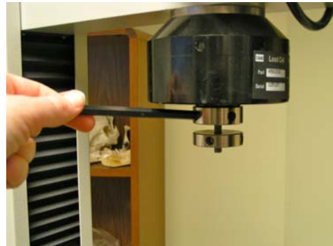
Fig. 24 Attaching tandem piggyback adapter to 10 kN load cell
