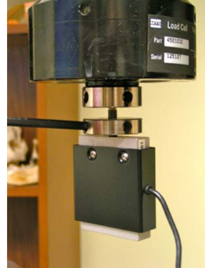
Fig. 25 (above) Attaching 25 N load cell to the tandem piggyback adapter
