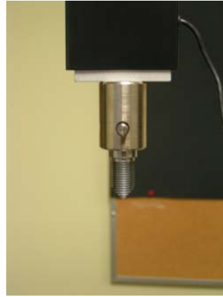
Fig. 28 25 N load cell, adapter, probe, and pin setup
