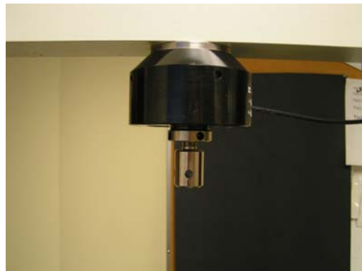
Fig. 42 (above) 10kN load cell with 10kN load cell adapter attached.
