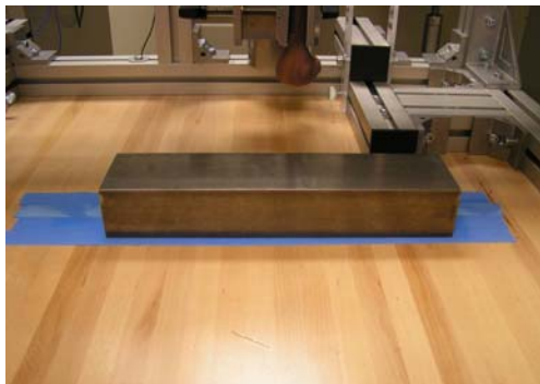
Fig. 51 Steel block is placed on top of four blue rubber tourniquet straps
