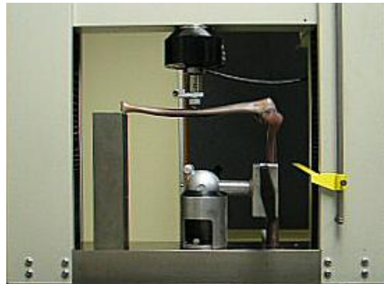
Fig. 44 Ulna bending during bending strength test.
